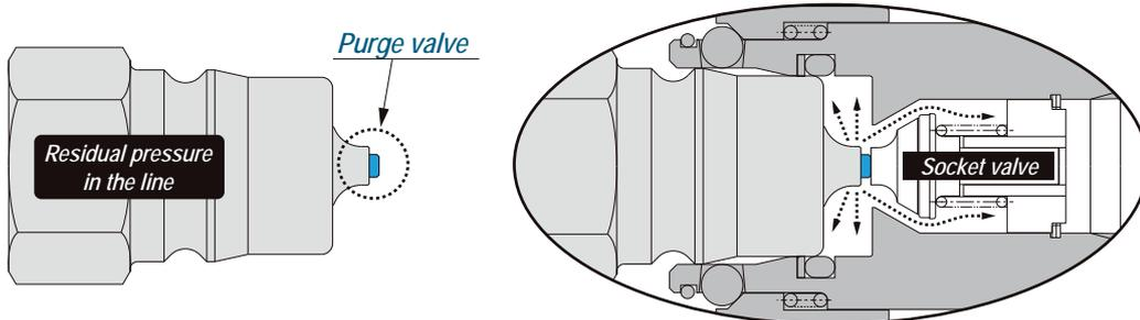
**Note:** Either socket or plug of HYPER HSP CUPLA must be used on the line where the residual pressure remains. The counterpart of HYPER HSP must be either plug or socket of standard HSP CUPLA. HYPER HSP CUPLA can be connected under the residual pressure in the line, but cannot during pressurizing. It may lead to incomplete connection, durability deterioration or possible valve fly out.
