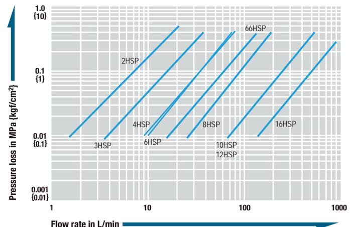
The flow volume of male thread type is increased by 5 to 10% compared with that of female thread type with conversion nipple.
