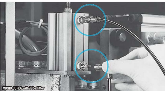
**Socket** SCB type (With Tube Fitter for panel mounting)
