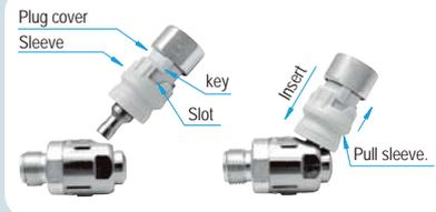
While keeping the plug inserted into the socket, tilt the plug so as to align the plug with the socket. Lock can be made by turning the sleeve.
