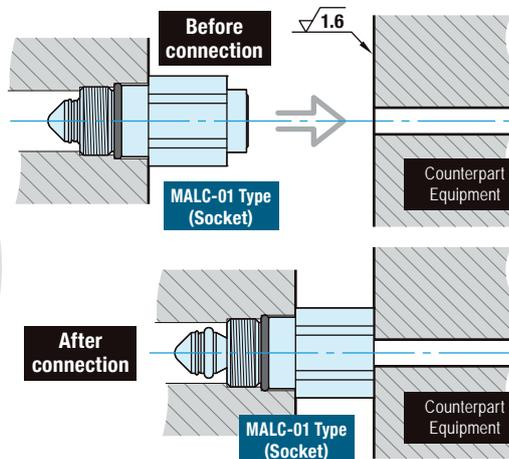
Distance between plates is 16 mm for solo use of socket.
