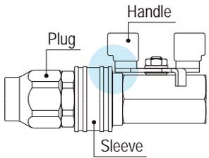
The handle of the ball valve locks the sleeve to prevent disconnection of the plug during use.
