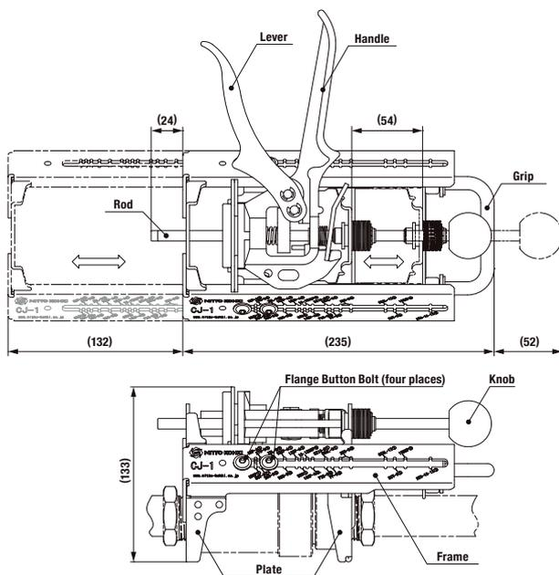
(Note) When the Handle is perpendicular to the body, it may interfere with CUPLA and will not be able to be used. In this case, tilt the handle to a convenient angle for use.
