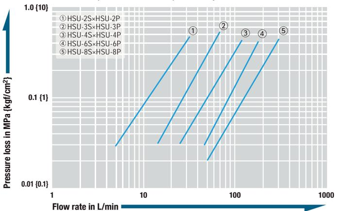
[Test conditions] - Fluid : Water - Temperature : 23°C±5°C
