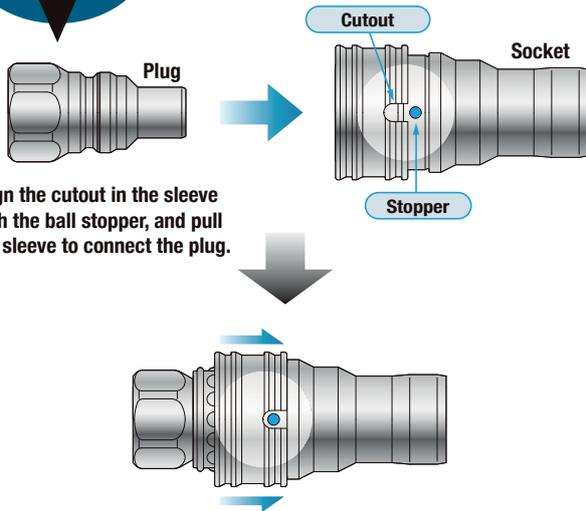
Align the cutout in the sleeve with the ball stopper, and pull the sleeve to connect the plug.
