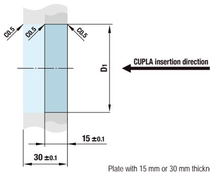
Plate with 15 mm or 30 mm thickness can be mounted.
