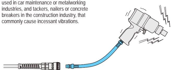
As an intermediate connection hose between “CUPLA” and a vibrating air tool.
