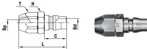
Grease is applied to the threaded part of stainless steel nut to prevent galling.
