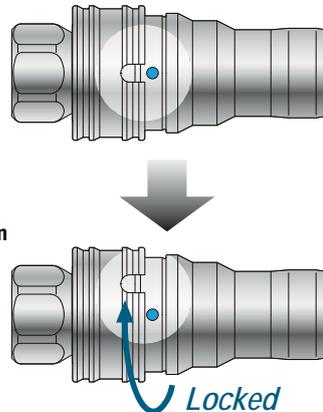
Without alignment of the cutout with the ball stopper disconnection cannot be made.
