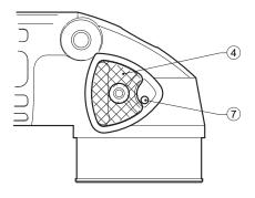
**3** Perform a trial run and wipe off extra grease that seeps out
