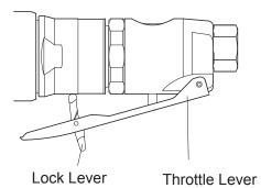
2 Hold the tool and while pressing the Lock Lever (1), press the Throttle Lever (2)
