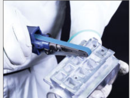
Chamfering of straight parts
