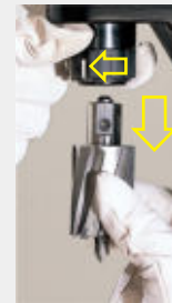
Removing the cutter
