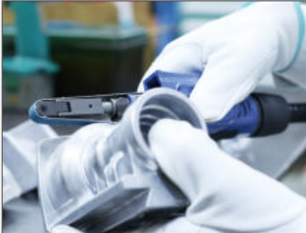
Deburring of die cast parts
